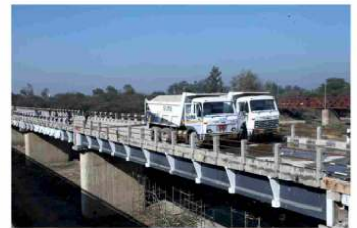
● Full Scale Load test for IRC 70 R load
